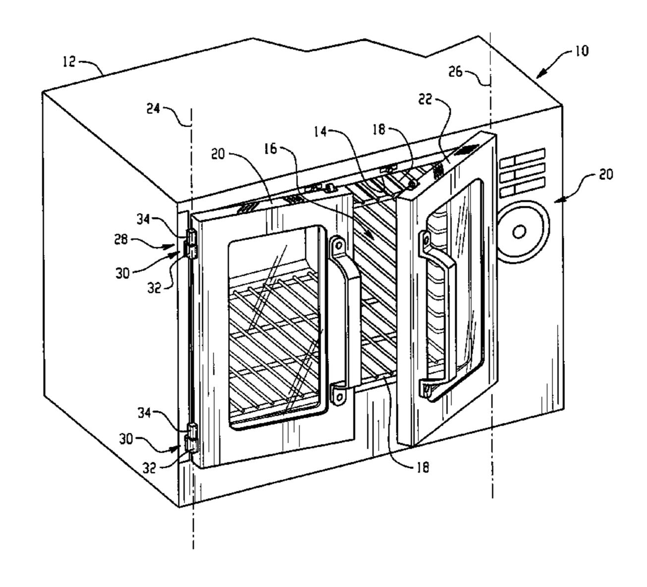
movement of the door assembly and upon separation of the pivot part of the door assembly from the pivot part of the housing the door becomes completely removed from the housing to enable the door assembly to be taken to a washing station for cleaning.
