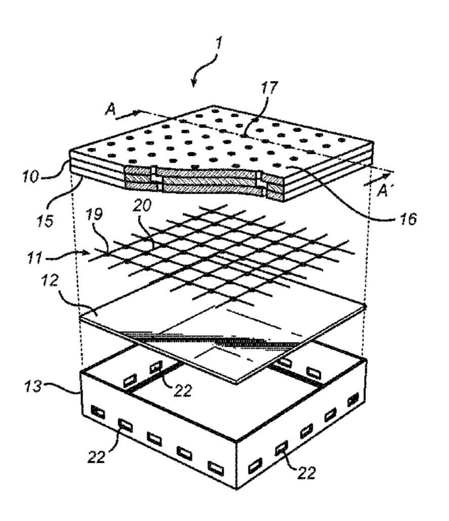
the hole on the optically reflective side of the soundabsorbing element will be prevented from passing through the sound-absorbing element.
