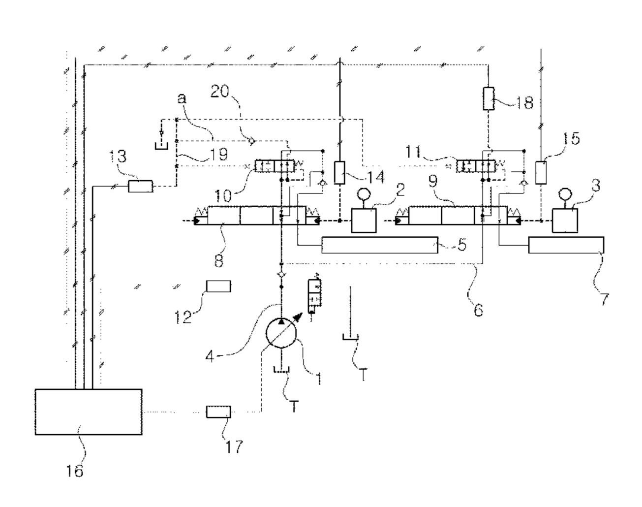
load sensing pressure line, and a control unit controlling a discharge flow rate of the hydraulic pump, wherein the system is configured so that the swing load pressure is not connected to the first pressure compensation valve on the attachment side when a combined operation of the swing device and the attachment is performed.
