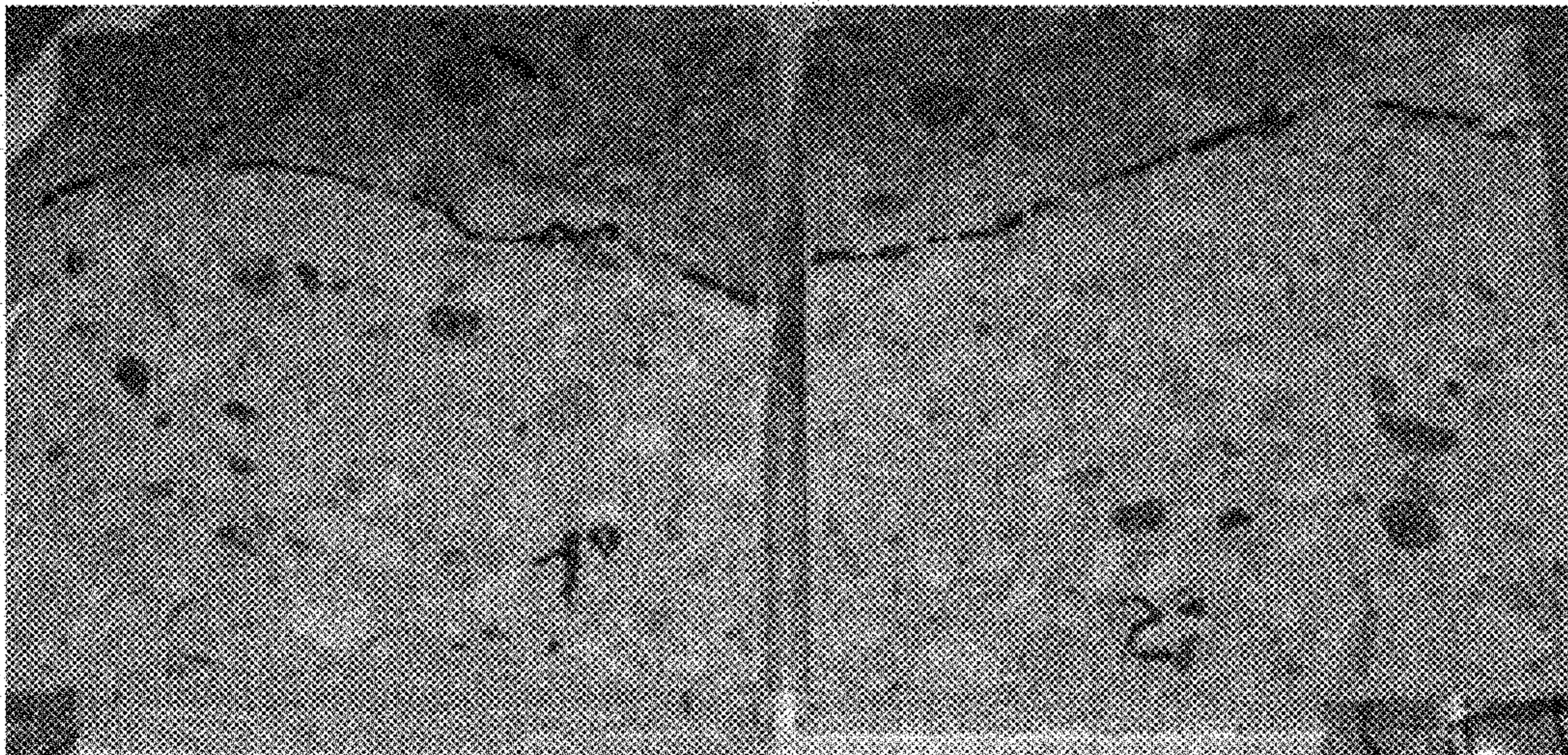
Figure 9. High-pressure water penetration test in a concrete specimen prepared without the accelerator described in Example 5-10 of the present invention (Example 19).
