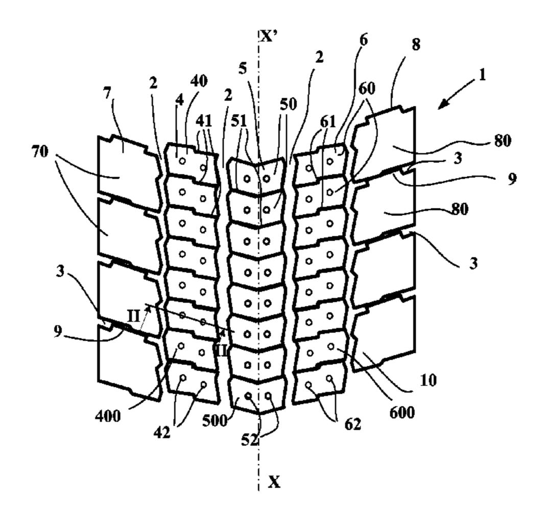
contact surface, having a depth at least equal to half the depth of the grooves, and determined such that it remains open as it passes through the contact patch so as to allow any liquid present on the road surface to be picked up.
