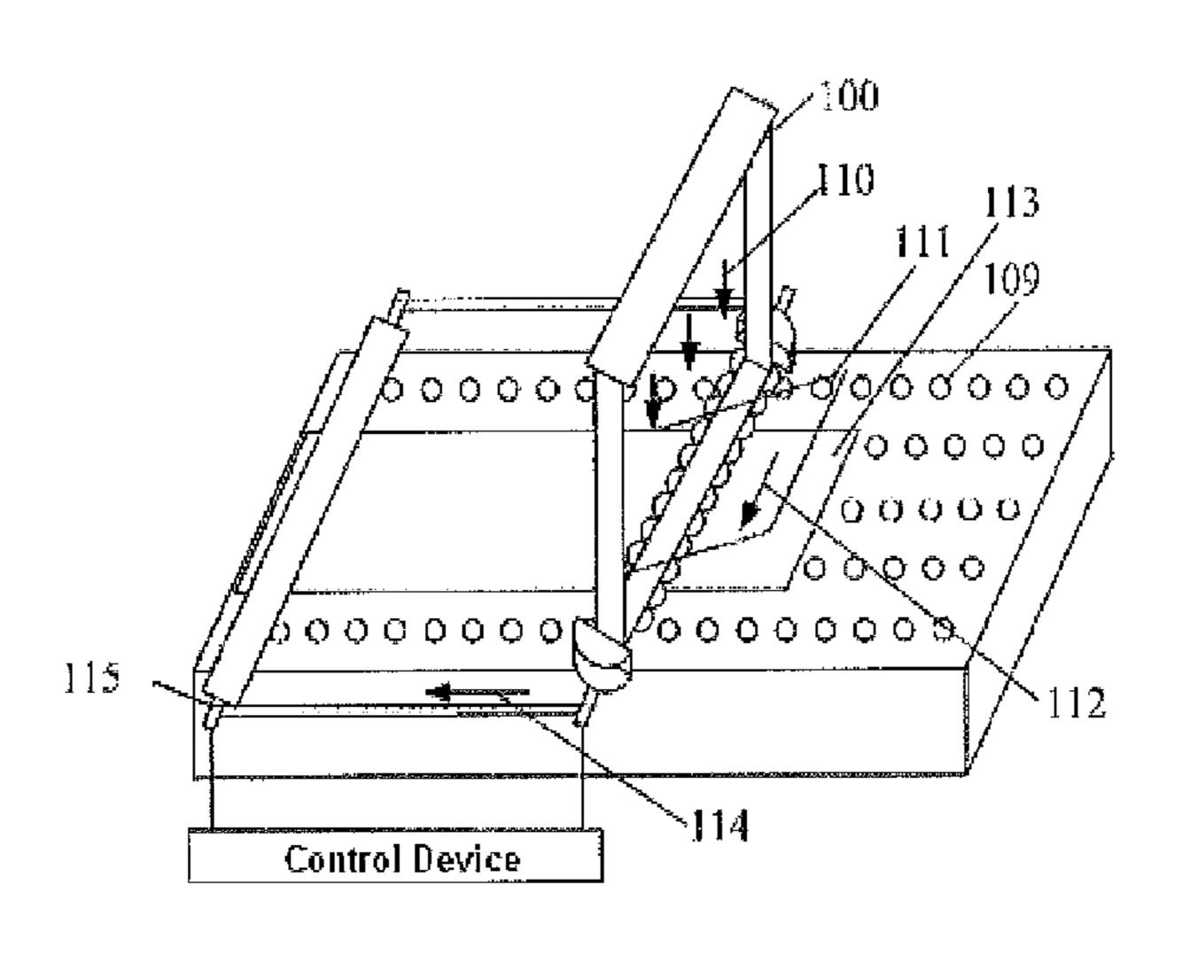
a cutting device arranged on the carrying device and configured to cut the adhesive so as to remove the touch panel from the display panel.
