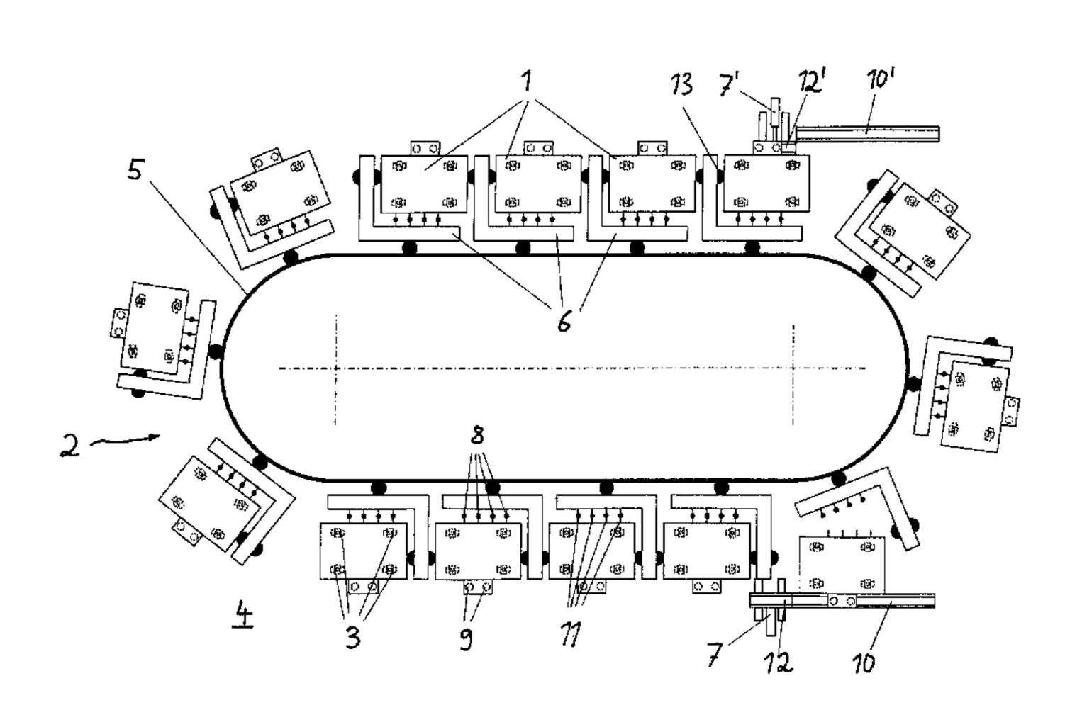
for taking the mould carriage (1) out of the production line (2), wherein here the mould carriage (1) is moved with its roils (3) on the stationary ground (4). Furthermore, the invention relates to a respective device.
