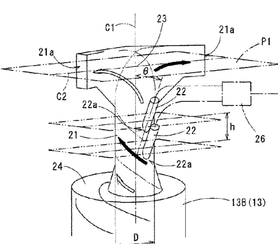
ing ports 22a of the material-supplying pipes 22, and D is a diameter of the duct 21, a ratio H/D is set to 1.4 to 2.5.
