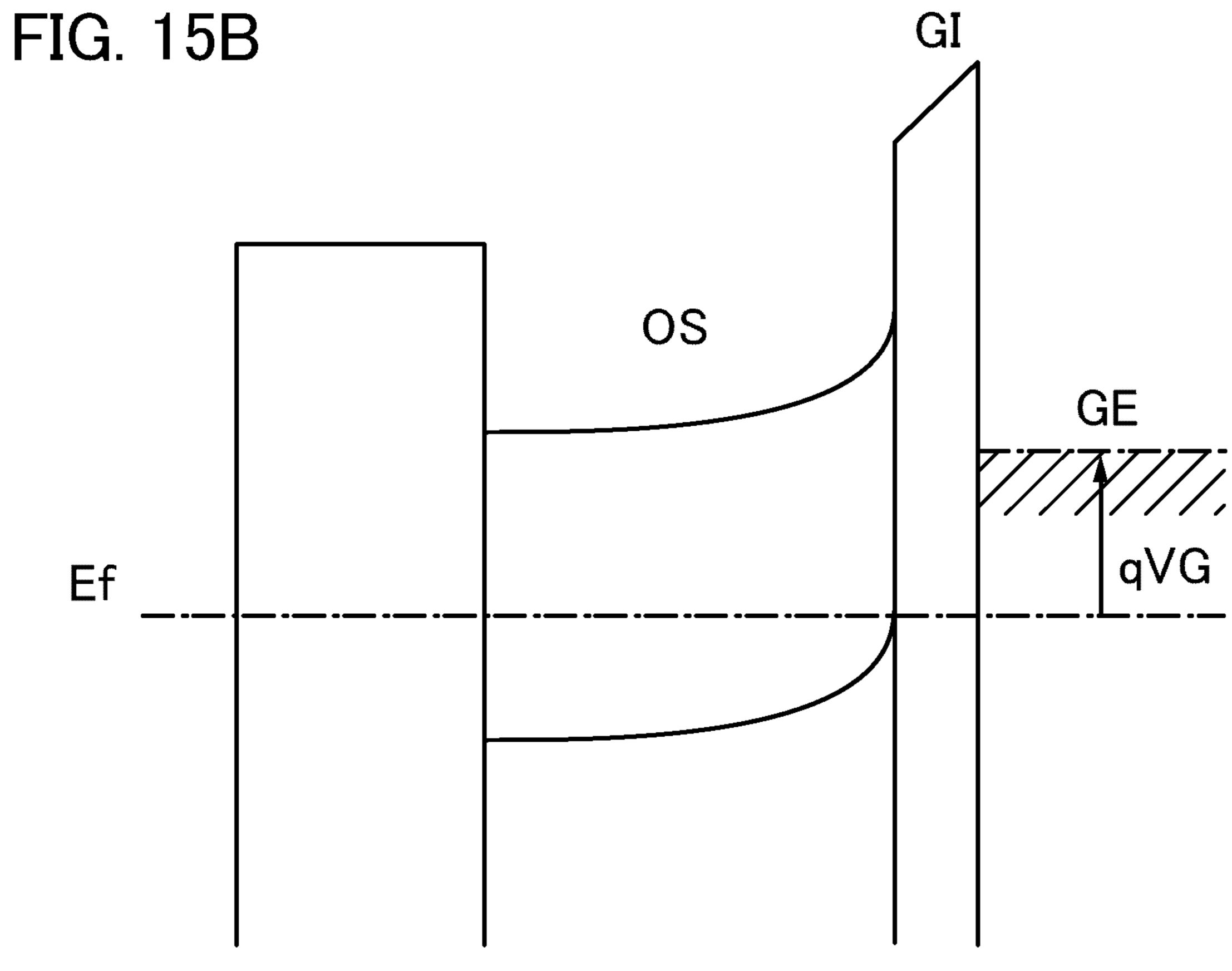
Energy band diagram along the cross section B-B' (VG<0)
