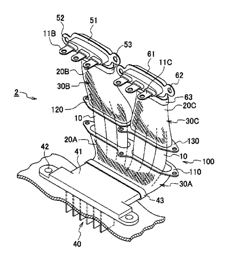
provided at each of the end portions of the branch line side braided wires (20B, 20C) for mounting the end portion of the main line side braided wire (20A).
