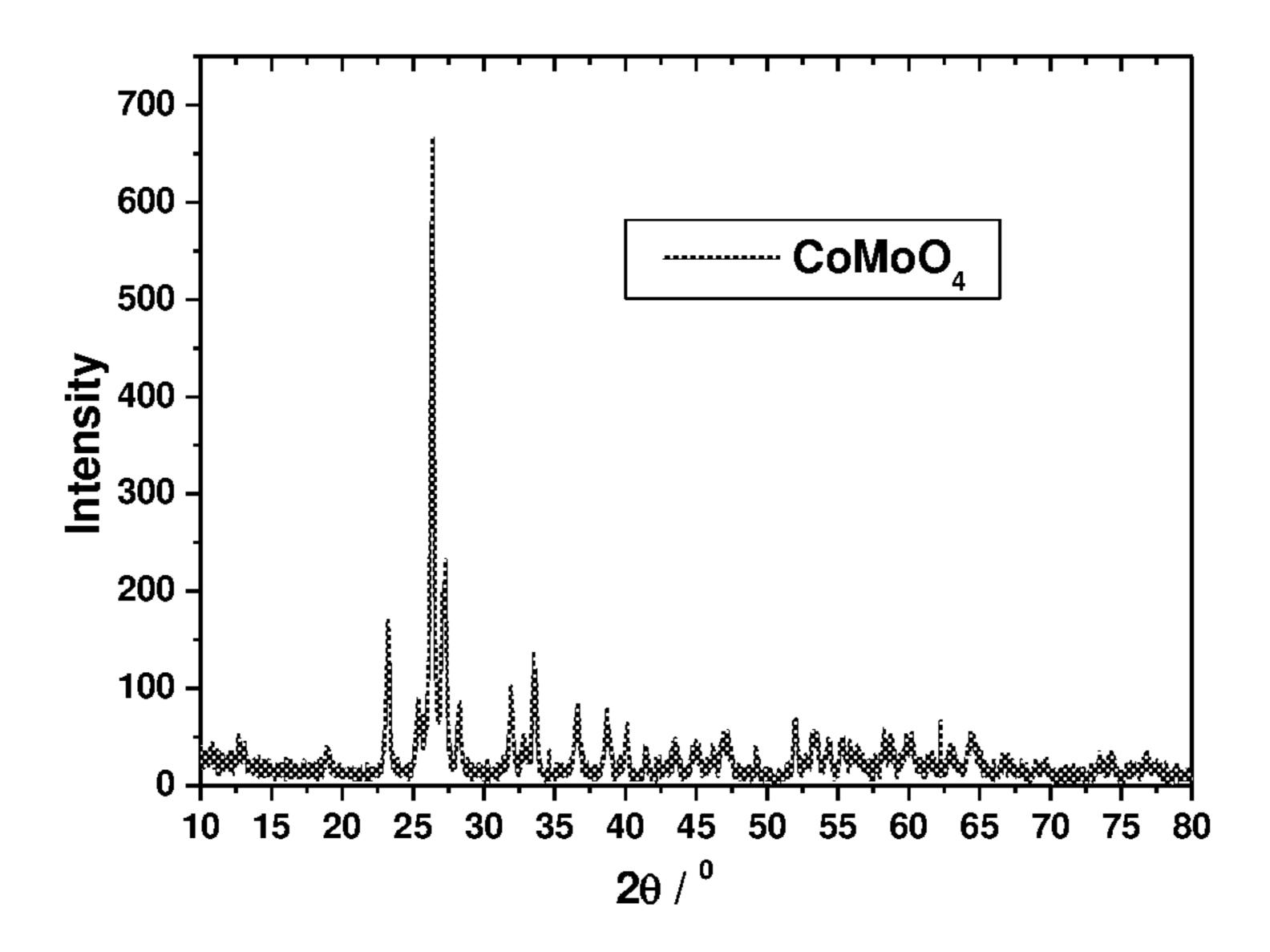
Figure 3: X rays diffraction pattern of the obtained cobalt molybdate CoMoO<sub>4</sub> according to the JCPDS card number JCPDS #21-0868
