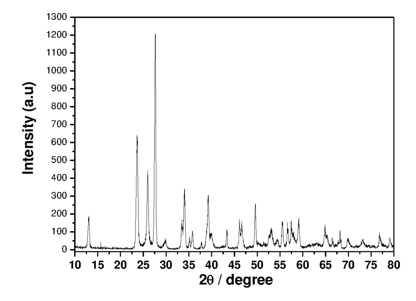
Figure 1: X rays diffraction pattern of  $MoO_3$ (JCPDS: 85-2405) obtained using the oxalate precursor.
