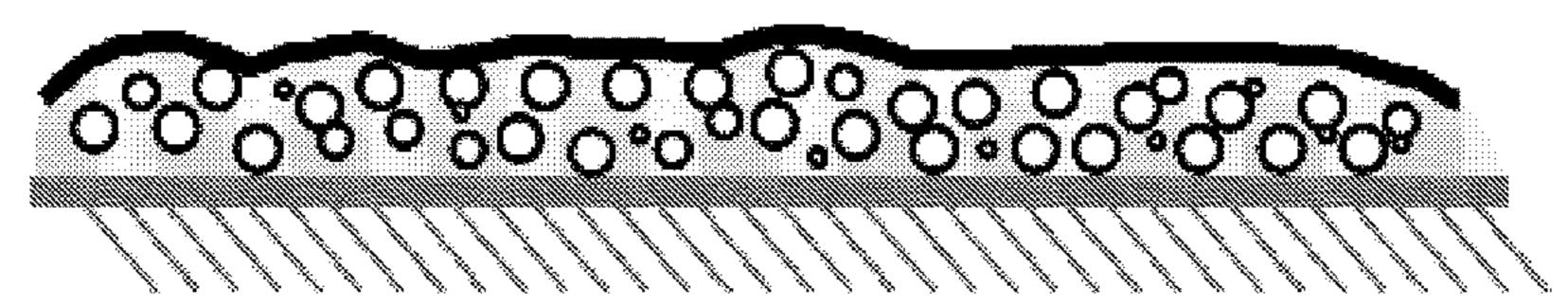
Taggant Capsules on Substrate with Barrier Layer
