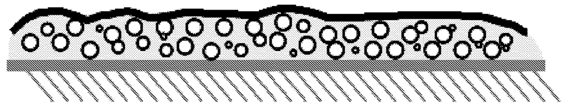
Taggant Capsules on Substrate with Barrier Layer
