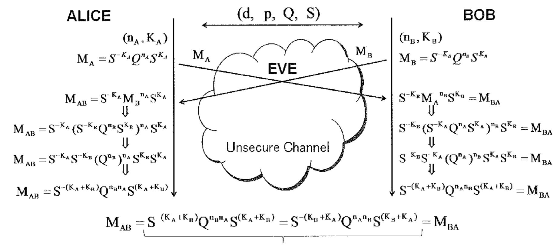
key by a shared secret key computation section. An encryption/decryption device is thereby capable of rapid generation of the secure common secret key.
