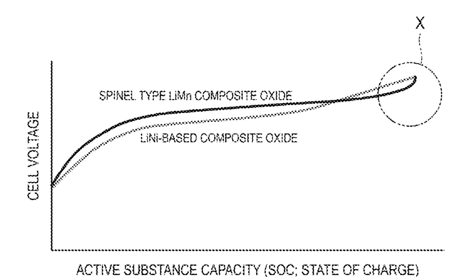
from non-uniformity of voltage across an electrode plane in a high-capacity and large-area non-aqueous electrolyte secondary battery that includes lithium nickel-based composite oxide as a positive electrode active substance.
