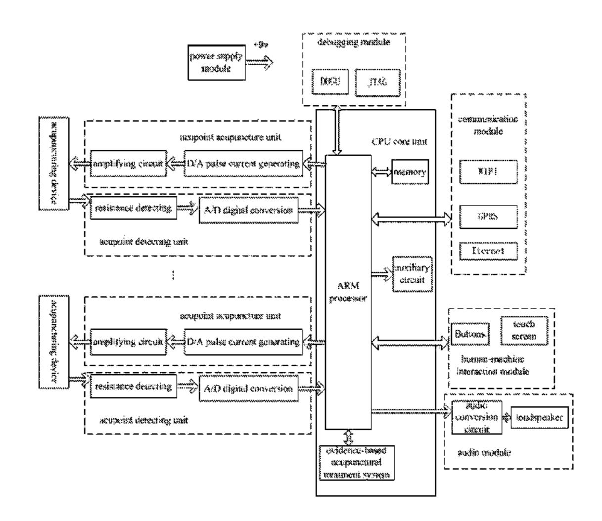
acupoint detecting unit comprises a resistance detecting circuit and an A/D digital converting circuit. The acupoint acupuncture and moxibustion unit comprises a D/A pulse current generating circuit and an amplifying circuit. The CPU core unit comprises an ARM processor, a memory, an auxiliary circuit and an evidence-based acupuncture and moxibustion therapeutic system, and the ARM processor is connected with the evidence-based acupuncture and moxibustion therapeutic system.
