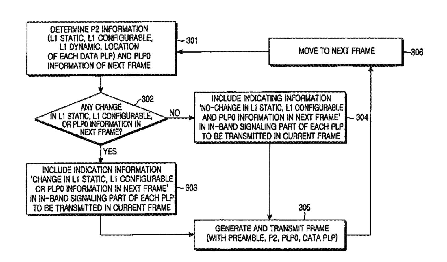
mation for the broadcast service in the next frame. Indication information, which includes information on a position in which the control information will change, is extracted from the frame and used to determine the position in which the control information will change.
