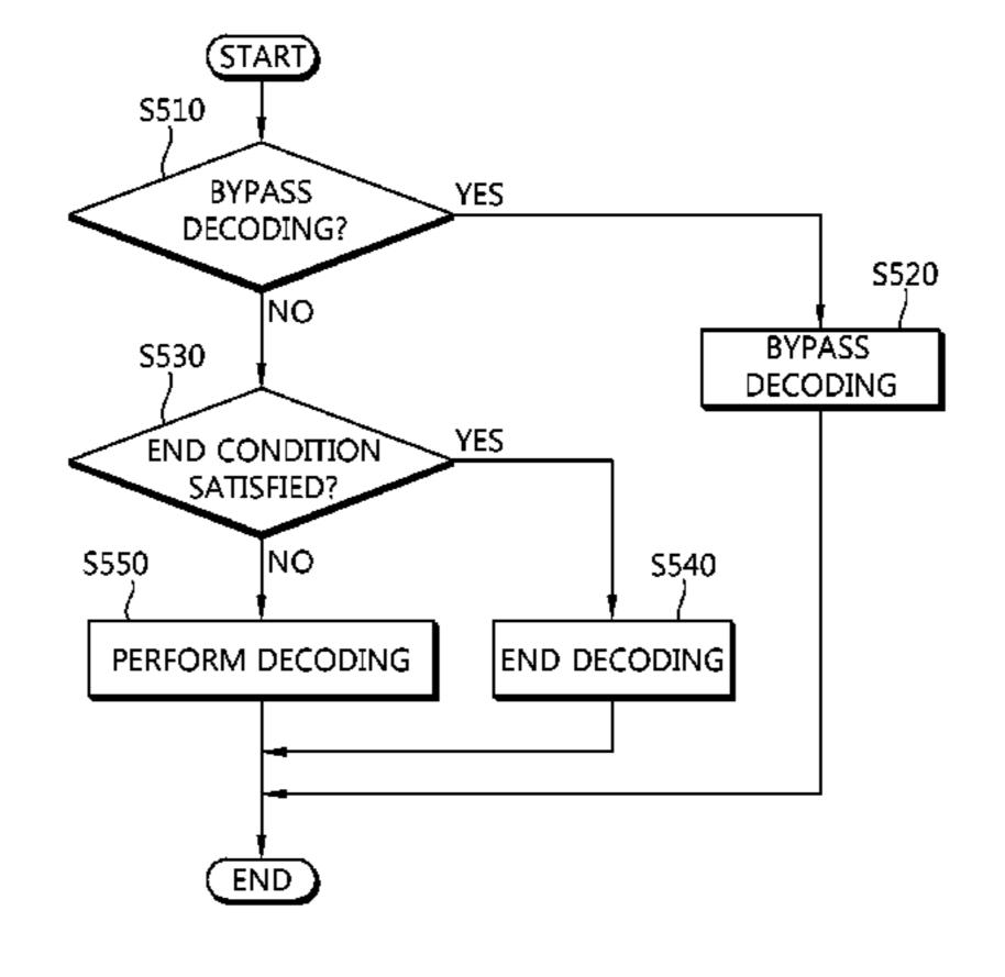
on the decoded bin. In the step of decoding the bin, context-based decoding or bypass decoding is performed for each bin of the syntax element.
