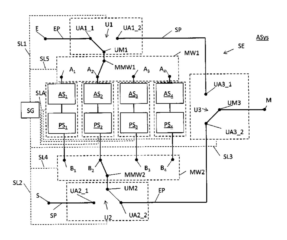
controller and a phase adjuster are connected between each connection of the number N of connections of the first multiple toggle switch and the second multiple toggle switch.
