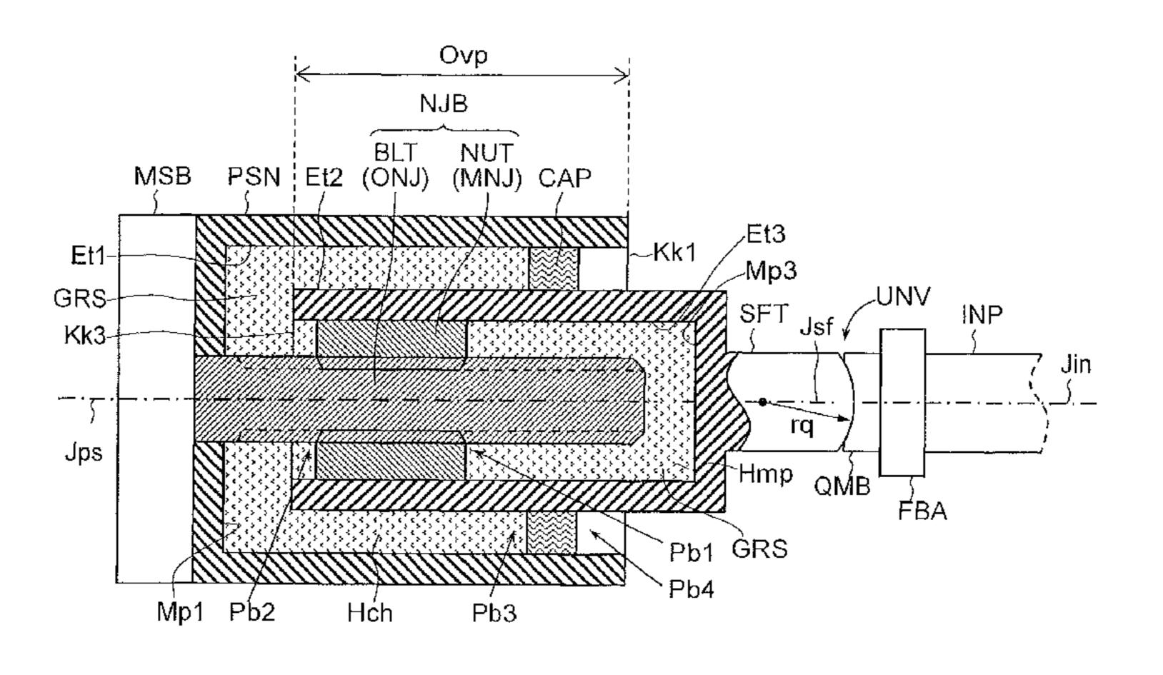
member partition a storage chamber connected to one end of the screw member, and a lubricant for lubricating the screw member is filled inside the storage chamber.
