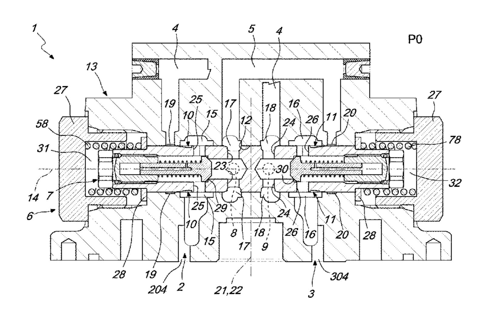
element that can move from an open position to a closure position. The first and second check valves respectively are provided with first damping means and second damping means in order to slow down the passage movement respectively of the first flow control element and of the second flow control element.
