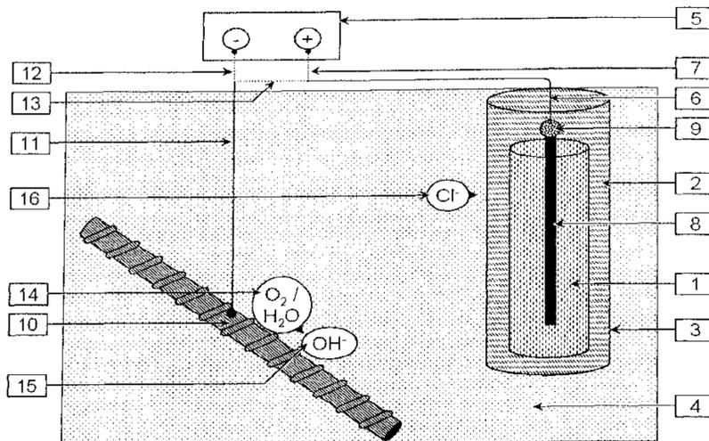
and activating the anode. Cathodic prevention is them applied. This is preferably sacrificial cathodic prevention that is applied by disconnecting the power source and connecting the activated sacrificial node directly to the steel.
