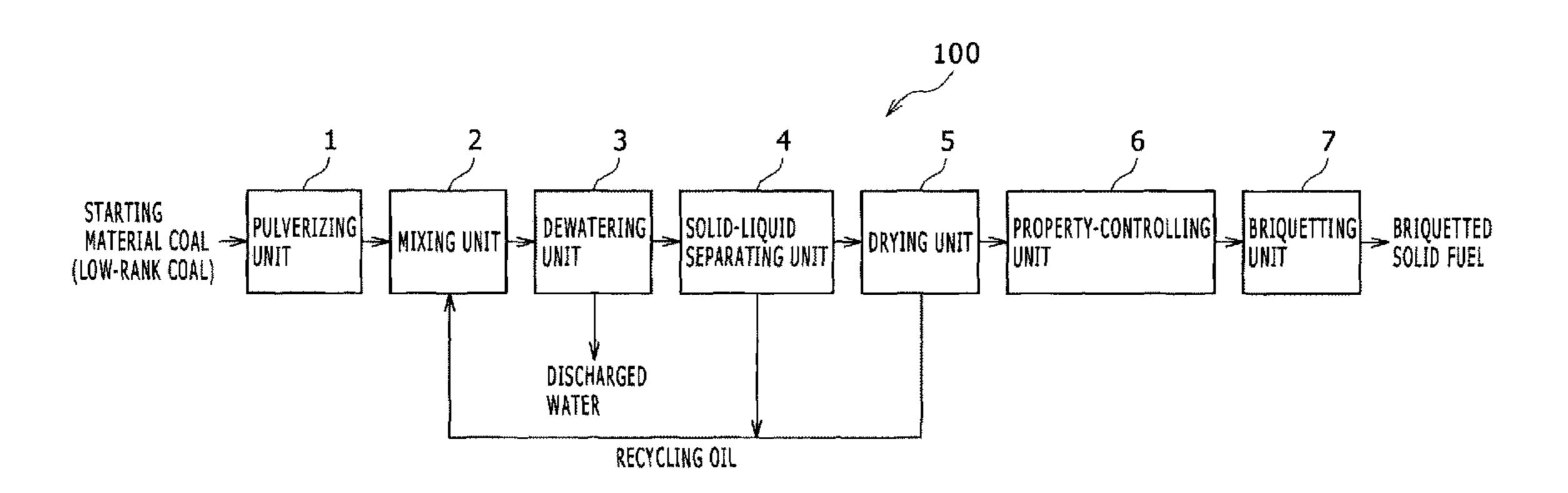
mass of the briquetting feedstock. The briquetting feedstock is briquetted under pressure to give the briquetted solid fuel in briquette form.
