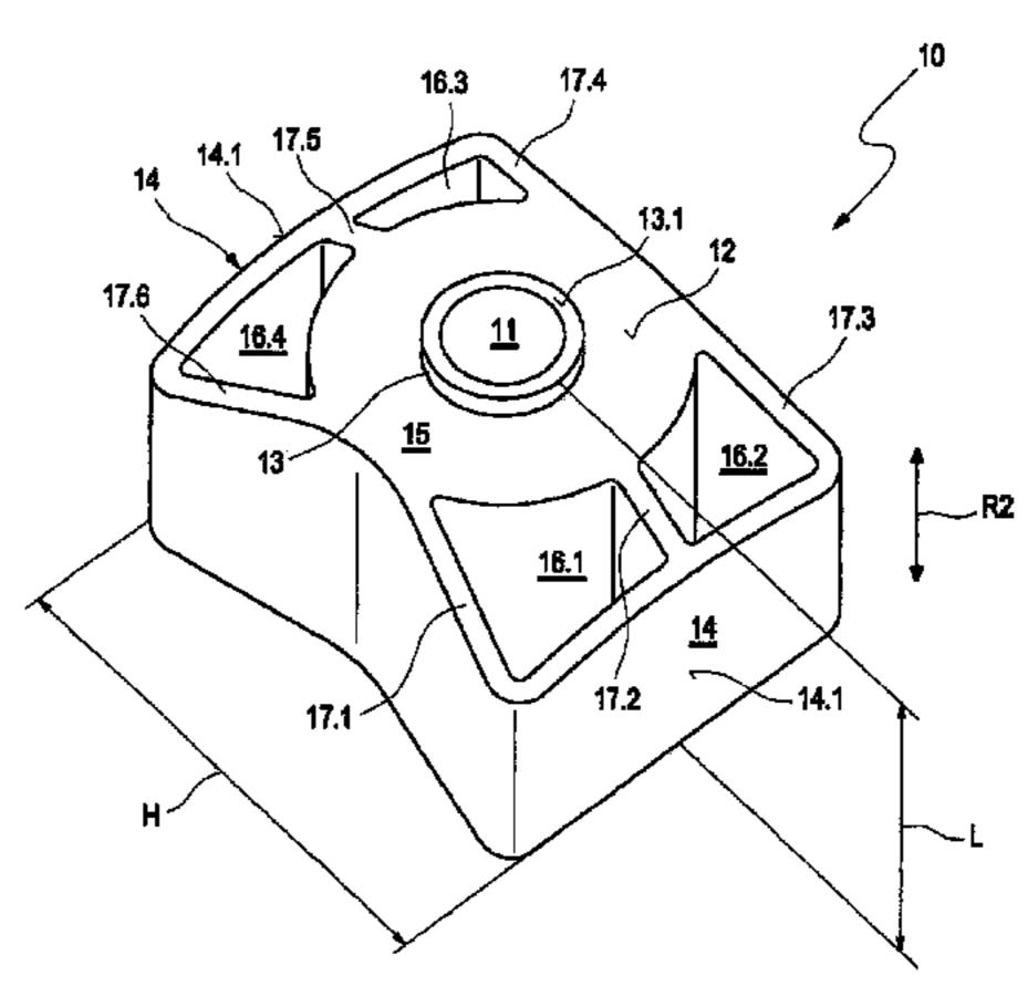
through opening in the boundary wall. The insert part is formed with a length in the profile direction of the insert part so as to enable insertion of the insert part into the chamber of the hollow profile and for positioning the same in the mounting position.
