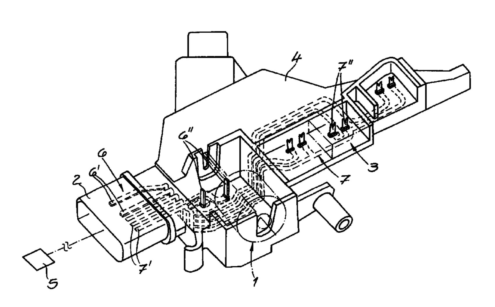
comprising a carrier element and a conductor track structure of individual metallic conductor tracks, which can be connected to the carrier element, wherein the conductor track structure is composed of at least two conductor track partial structures, each having a different material thickness, of the associated conductor tracks.
