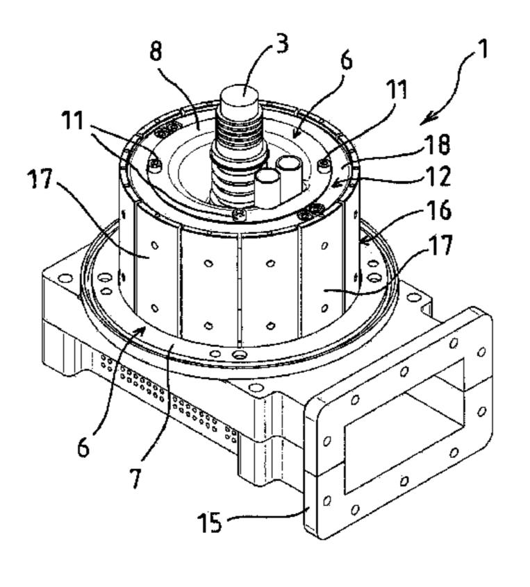
magnetic field generation apparatus, and the old magnetron tube is removed from the magnetron and replaced with the new magnetron tube in order to then remove the diverting element again.
