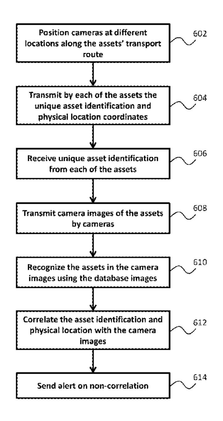
server is configured to recognize the assets in the camera images, to correlate the asset identification from the receiver with recognized assets in the camera images, and to correlate the physical location coordinates of each of the assets with physical location coordinates of the cameras. The system monitors the visual appearance of the assets, and keeps track of whether or not they have sustained physical damage.
