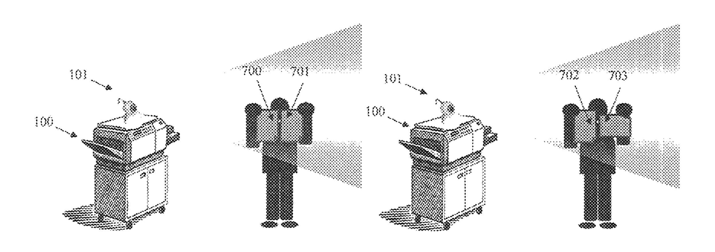
portion executes the processing of the document sheet image data based on the operation corresponding to the operation image data when it is determined that the document sheet image data and the operation image data are contained in the photographic image data.
