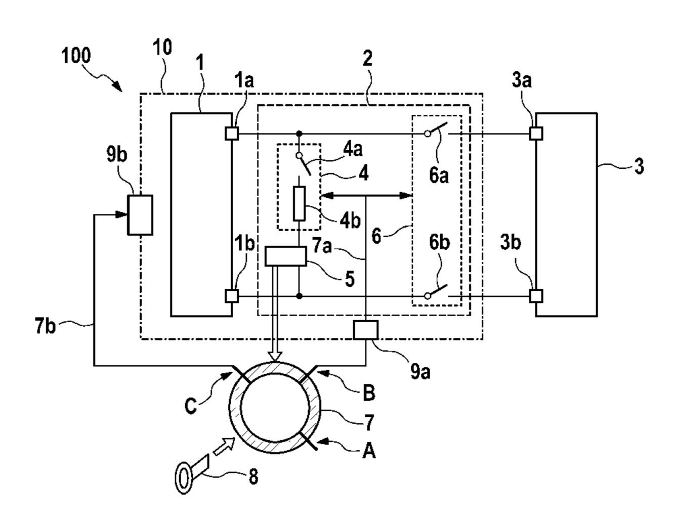
tion of the safety switch, and having a monitoring device which is designed to monitor electric parameters of the discharge circuit or of the high-voltage components, and to release the lock of a housing for the high-voltage components if at least one of the electric parameters of the discharge circuit or of the high-voltage components falls below a predetermined threshold value.
