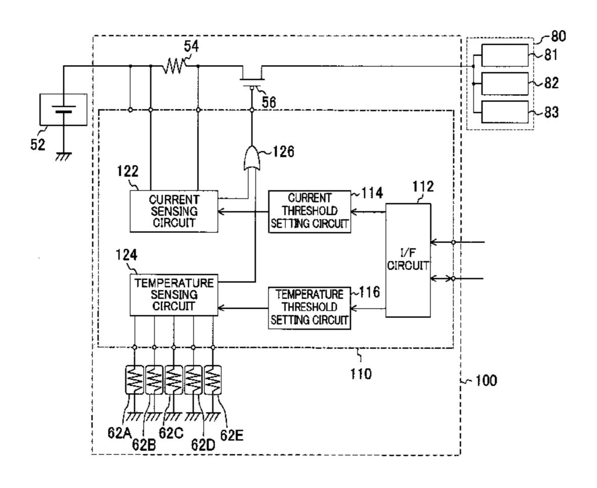
control circuit which generates a clock signal including pulses with a predetermined period. The sensing circuit determines the current or the temperature of the sensing element during an active period of the clock signal.
