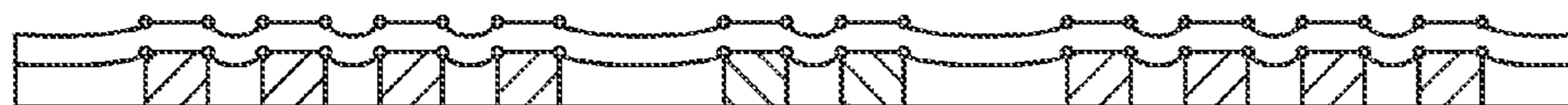
AFTER BOTTOM DIELECTRIC DEPOSITIONS
