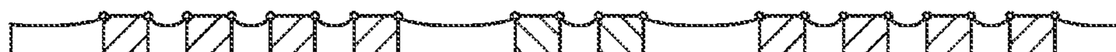
AFTER CMP (SHOWING DISHING AND BUMPS)
