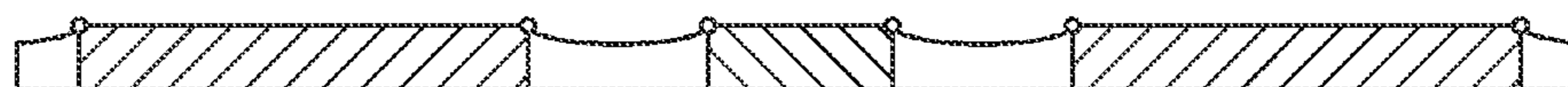
AFTER CMP (SHOWING DISHING AND BUMPS)
