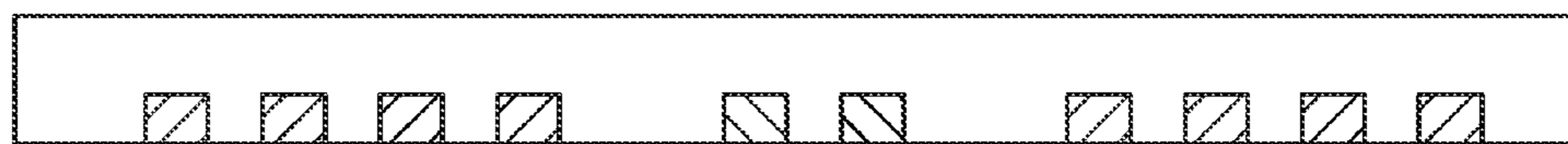
ELECTRODES + FILL DIELECTRIC DEPOSITION
