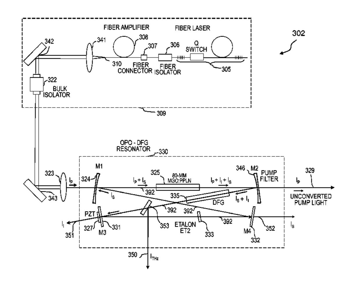
beam-extraction mirror, and an  $I_S$ -beam-extraction mirror, and a fifth  $I_{TH_Z}$ -beam-extraction mirror.
