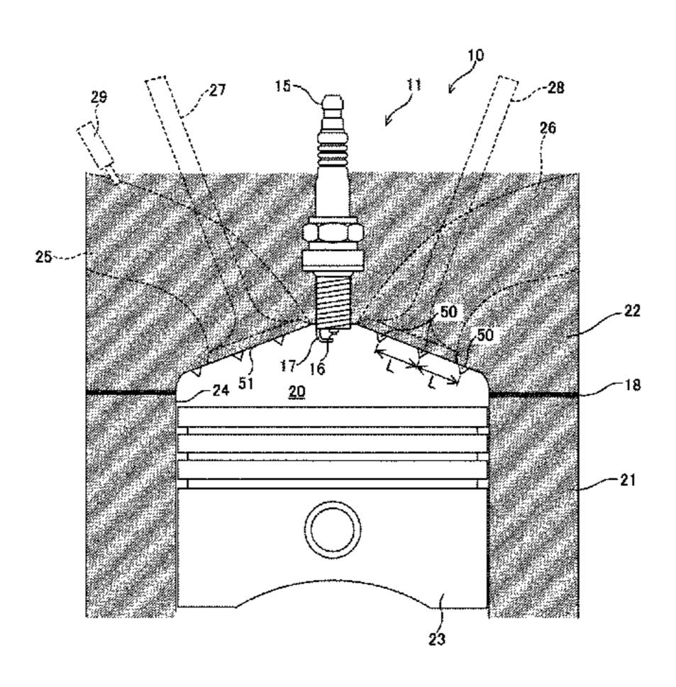
ing from a partitioning surface that partitions the combustion chamber. At least a part of the protruding member is made of a conductor.
