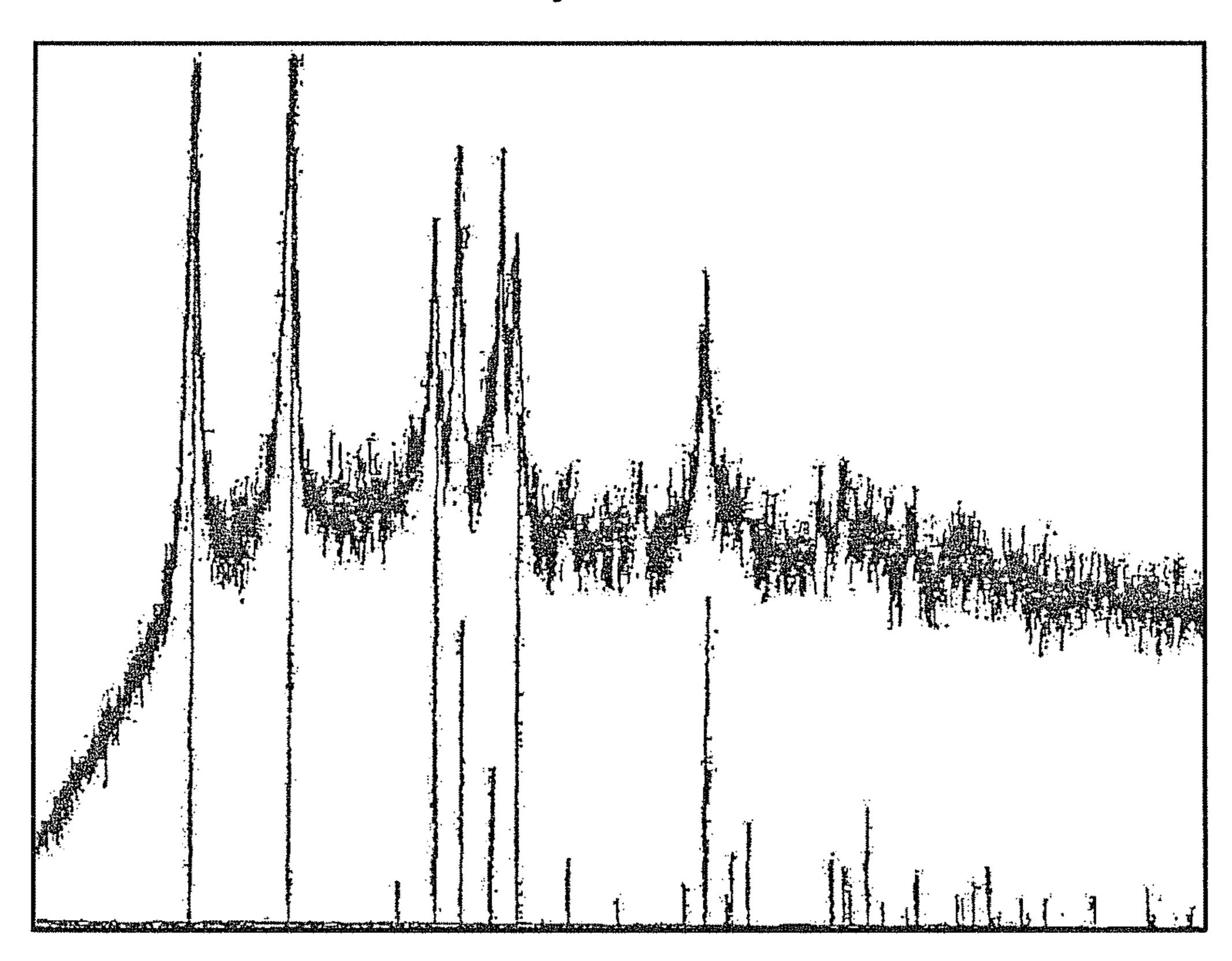
Shows that the particles are  $Cu(OH)_2$  with no iron oxide or hydroxide peak, indicating that the  $Cu(OH)_2$  is doped with iron.
