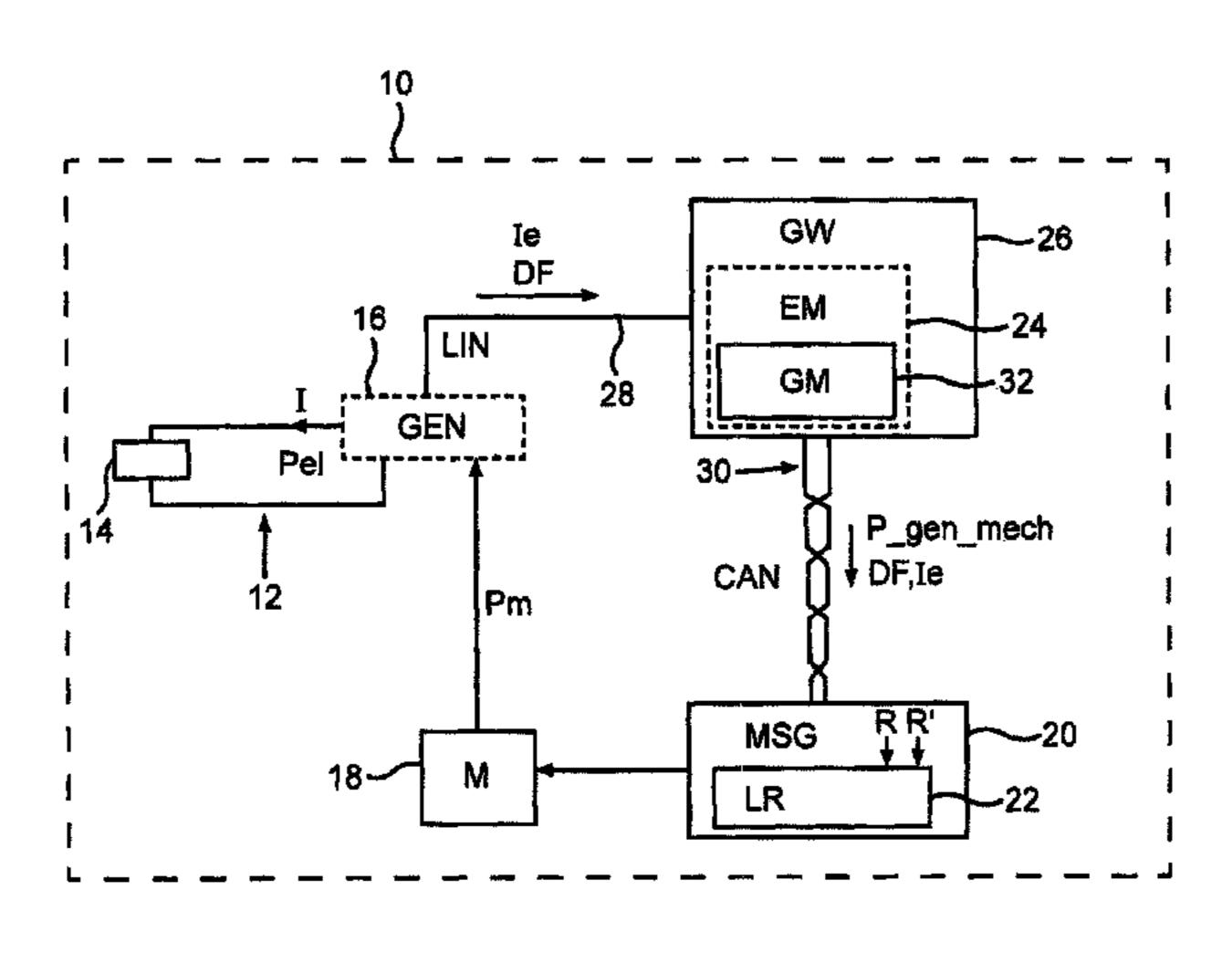
the energy management unit and dependent on the relative change in the monitored operating variable.
