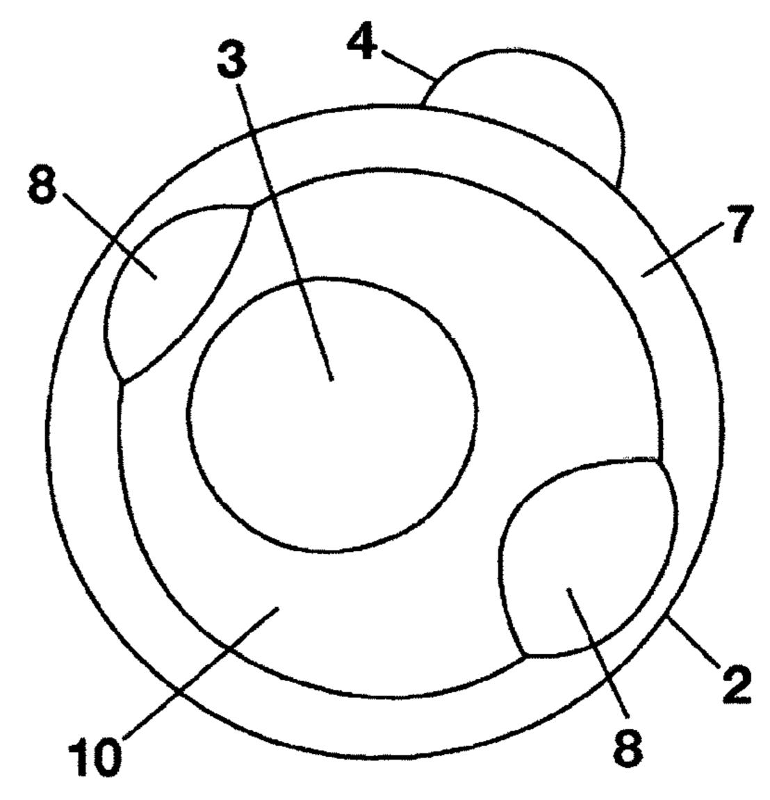
handle, and the outside barrel surface. A substantially circular brim serves as a surface transition between the inside and outside surfaces of the cylindrical barrel and can contain a plurality of substantially concave scoops, each centered approximately ninety radial degrees offset of the handle.
