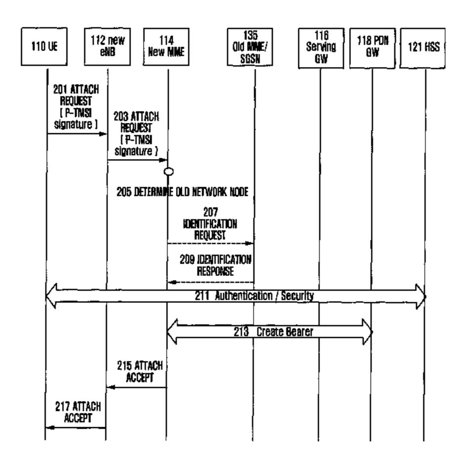
involvement a UE, an MME, and an old MME or an old Serving General Packet Radio Service (GPRS) Support Node (SGSN) to which the UE has been attached before so as to facilitate discovering a best node using the UE information acquired from the old MME or old SGSN during the communication between the UE and the network, resulting in a reduction of a communication delay between the UE and network and an improvement of communication efficiency.
