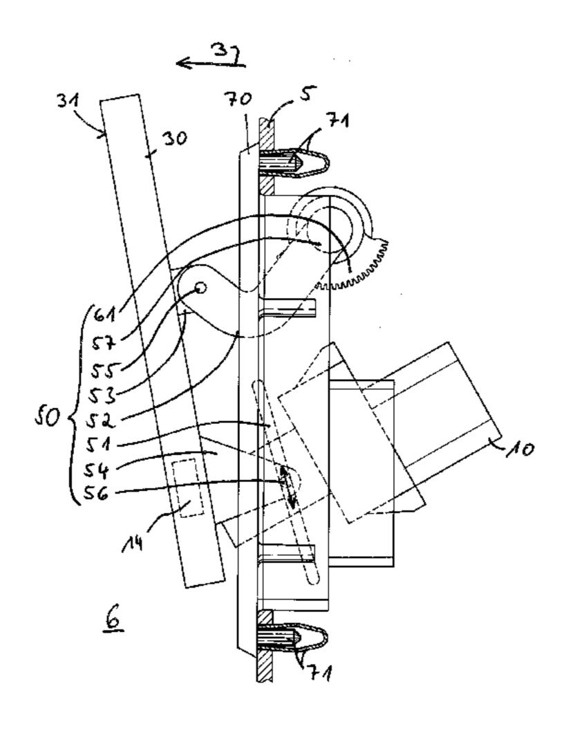
drive interacts with a mechanism in such a way that the outer surface is always in the exterior area of the motor vehicle in each position of the cover element during the movement of the cover element between the closed position and the open position.
