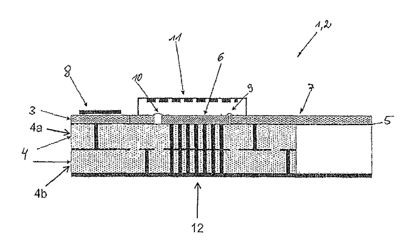
posed of a high-strength polymer material, which stabilizes the multipolymer circuit board, and a metallization layer, which is arranged between the first layer and the second layer and serves for shielding and for signal carrying, and the multipolymer circuit board carries the at least one millimeter-wave circuit and the at least one antenna.
