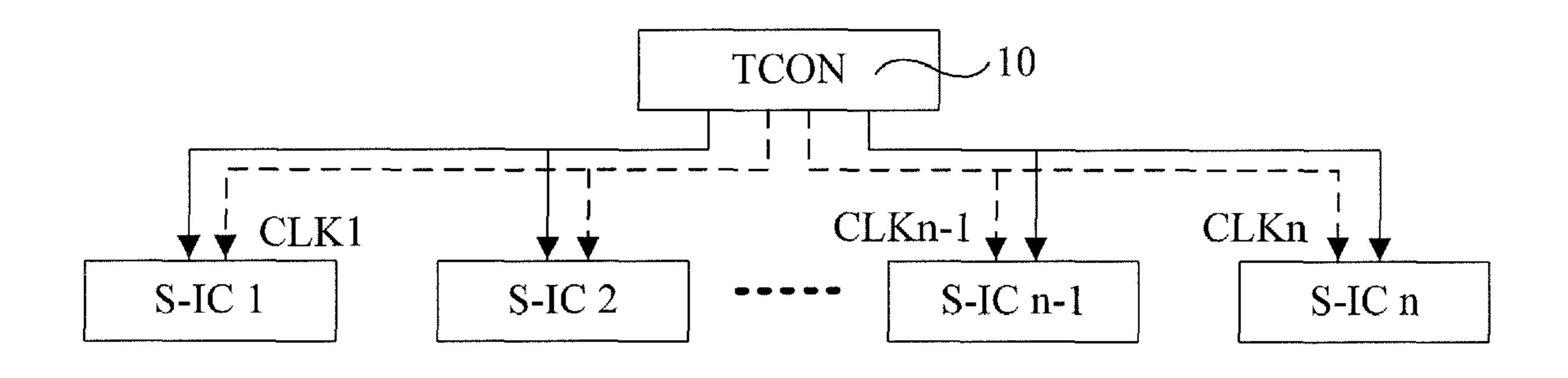
ing to the maximum delay time such that respective signal driving units (30) receive the second clock signal (CLK2) simultaneously. Therefore, delay errors of the display driving signals can be eliminated, and distortion of the display image can be avoided.
