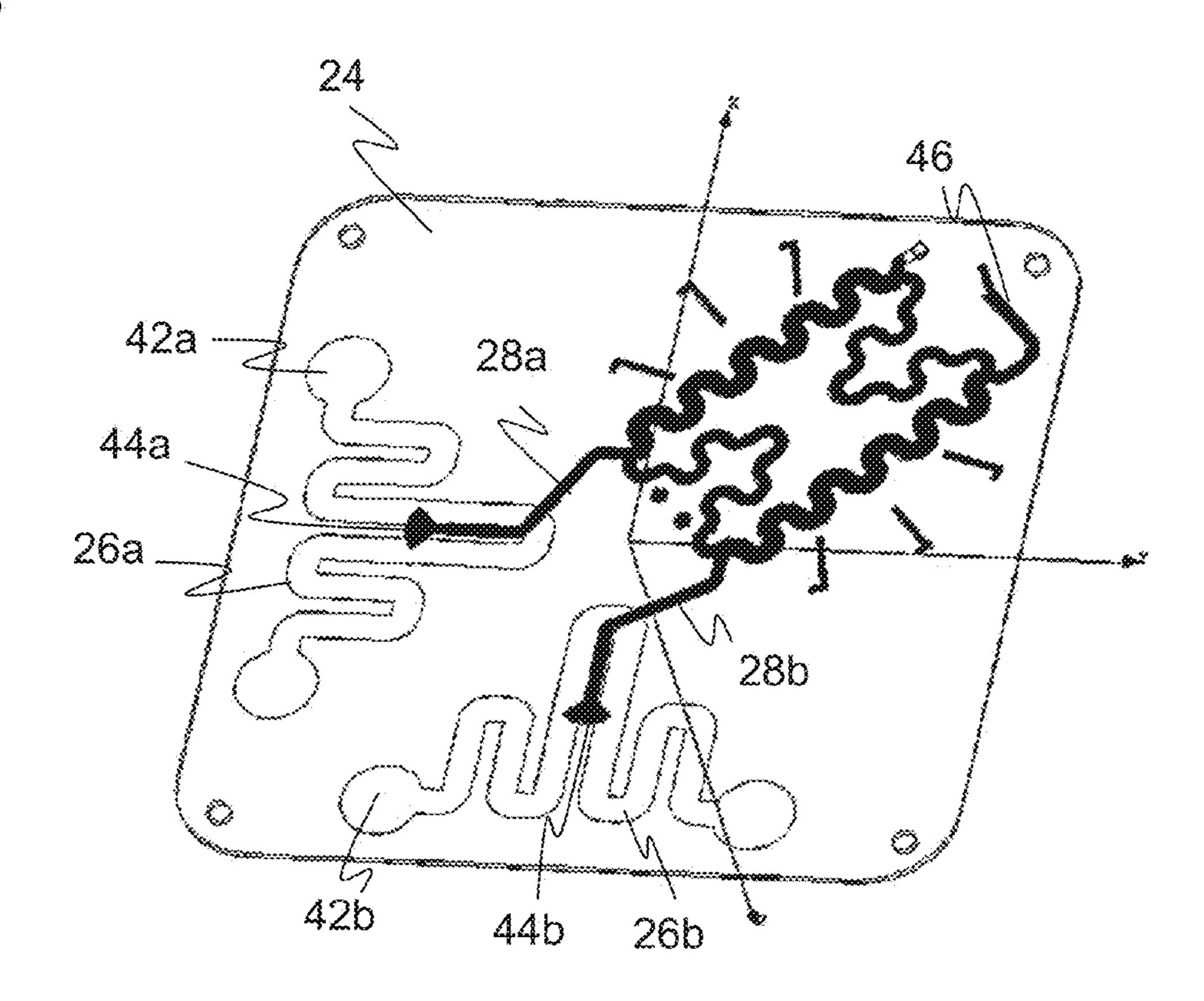
The invention relates to an antenna having a circuit board and a slot in accordance with the preamble of claim 1 as well
