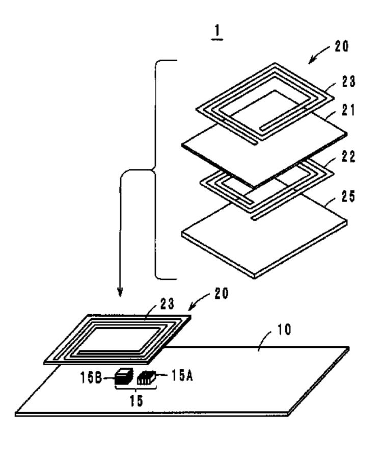
the second coil antenna does not overlap the coil conductors of the booster coil antenna as viewed in plan.
