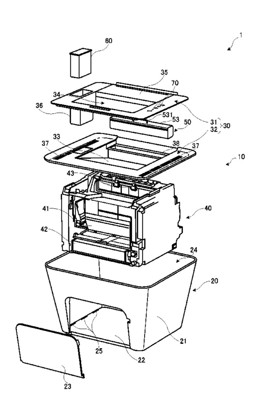
bottom in the housing body. When the lid is removed from the image forming apparatus and the image forming section is lifted above the opening, the image forming section is taken out of the housing body through the opening and the housing body is removed from the image forming apparatus.
