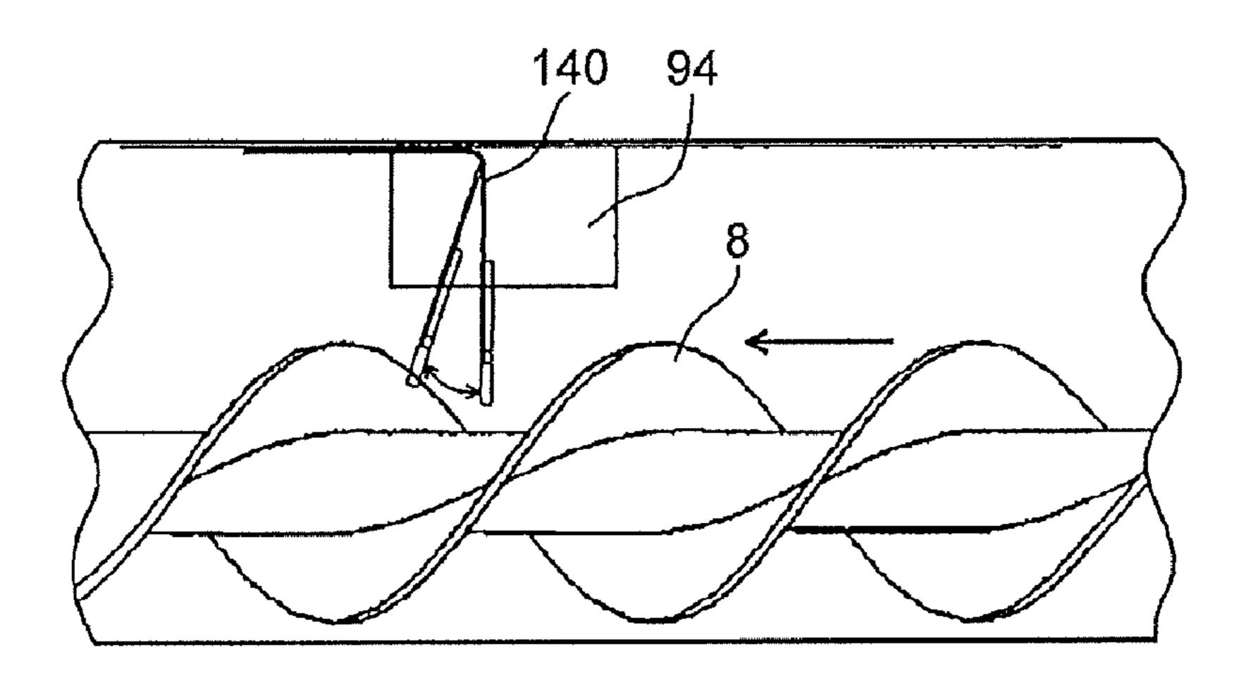
thereafter being elastically restored by being brought out of contact with the developer conveying member.
