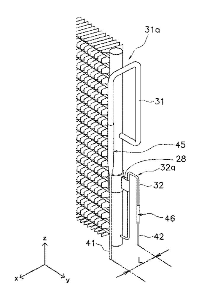
disposed in an area outside of directly under the connecting part of the aluminum gas pipe and the copper gas pipe.
