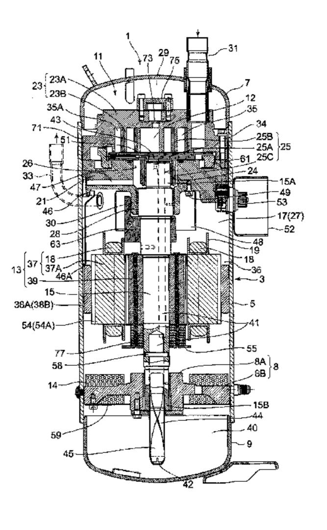
the driving shaft 15, and intercommunication paths 38B, 54A through which lubrication oil scraped up by the pickup 45 and supplied to respective lubrication sites is returned to the lower side of the driving motor 13 are provided between the stator 37 and the spacer ring 38 or between the spacer ring 38 and the casing 3.
