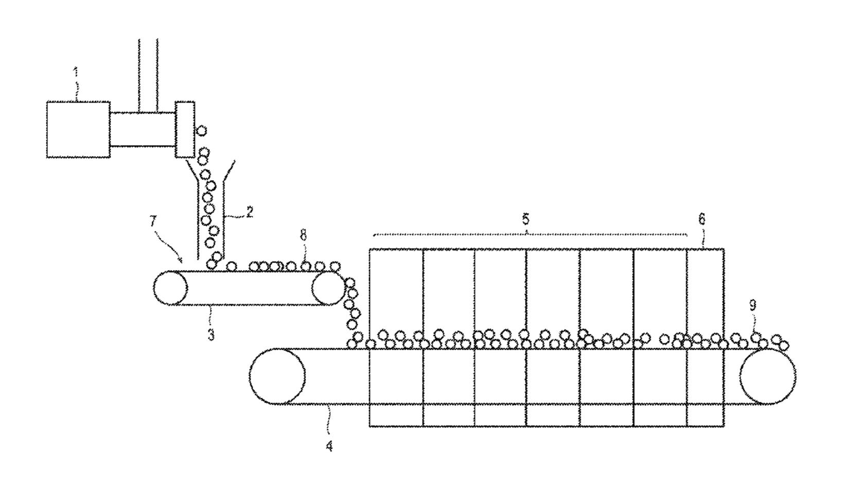
ous through-flow belt-type dryer by a traverse conveyor to dry the particulate water-containing gel-like cross-linked polymer, in which the belt temperature of the traverse conveyor is 40 to 120° C. and/or the water soluble component in the particulate water-containing gel-like cross-linked polymer on the traverse conveyor is 10% by weight or less and the water soluble component is increased after the drying step.
