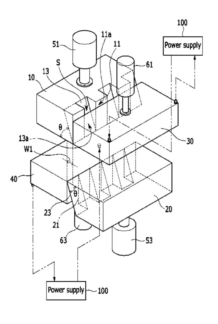
apply clamping force and load, wherein the metal plates are disposed between the upper shear bonding mold and heating clamper, and the lower shear bonding mold and heating clamper.
