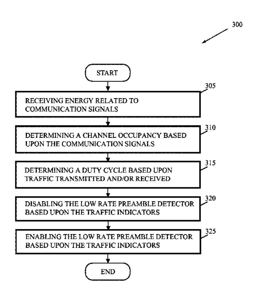
may determine whether to disable the low rate preamble detector. Further embodiments comprise logic to design a station, determining whether to include a low rate preamble detector based upon parameters related to channel traffic.
