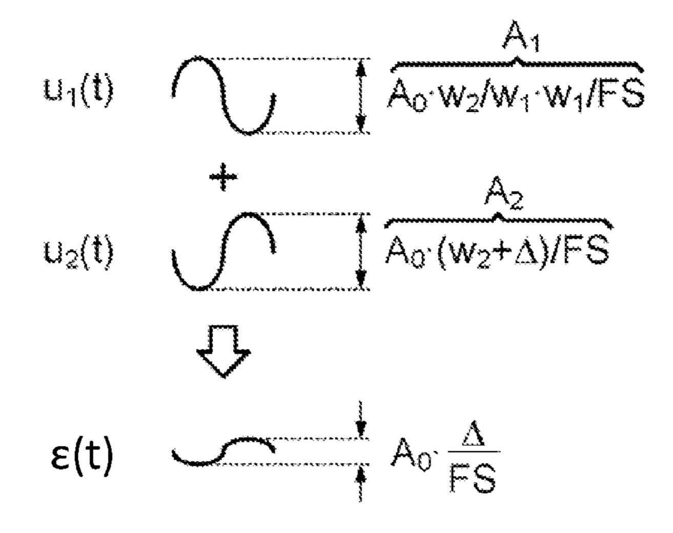
A<sub>0</sub> depends on noiseshaper dynamic range  $\rightarrow$  choose A<sub>0</sub> close to overload for max sensitivity
