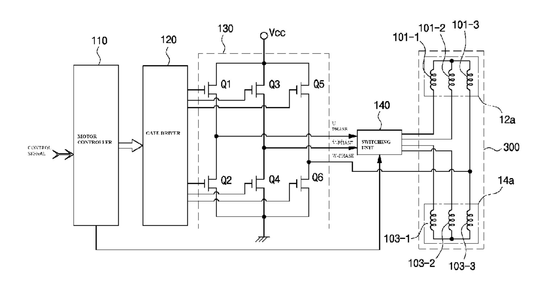
coils of the first and second U-phase, V-phase, and W-phase stator coils for the washing machine motor.
